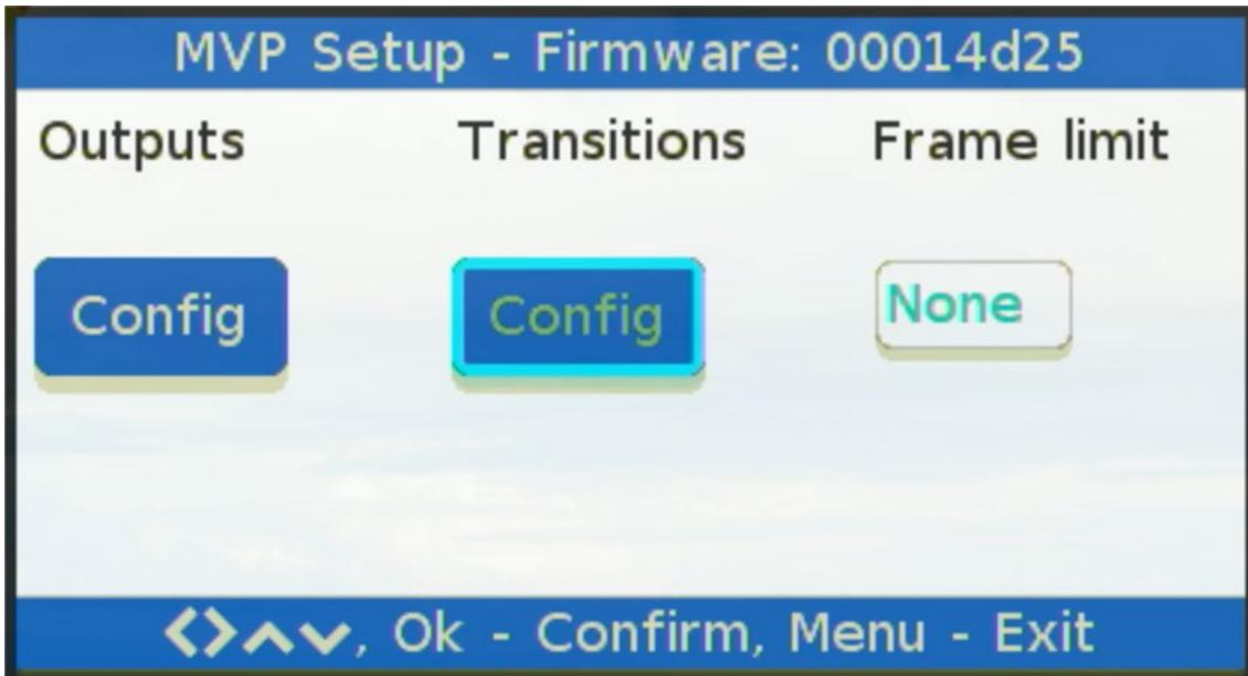
In the transition/configuration menu, the user can control the RATE, and thus determine the duration of the MIX and FTB effect.
