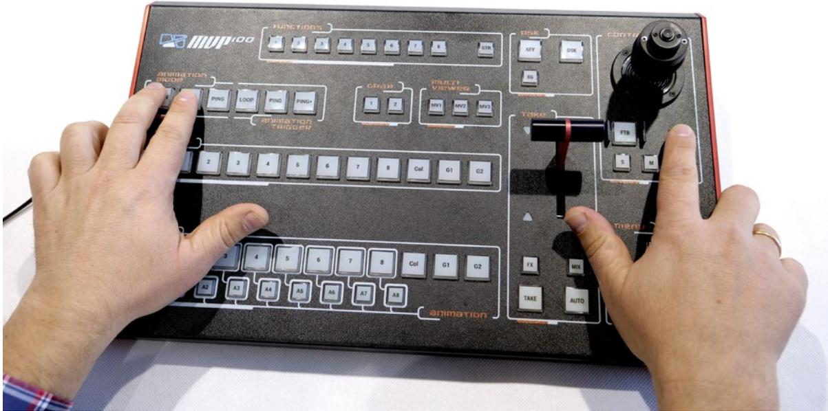
The keyboard shows the current brightness of the keys. Pressing TAKE key several times decreases the backlight's brightness. AUTO key increases brightness of the keys. Picture below
