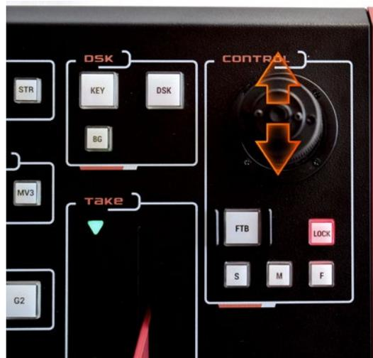
F4 is the JOYSTICK's knob calibration. We turn it several times to the right and to the left to the extreme positions. When you complete that, the F4 LED will light up in white. Picture below.
