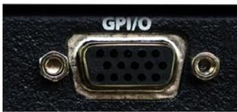
GPIO interface – a universal input/output port for various applications. GPIO (General Purpose Input/Output) is an interface used for communication between MVP-100 system components and various peripheral devices. GPIO pins can be used as inputs. Thanks to GPIO Interface it is possible to broaden MVP-100 device’s functionalities resulting from cooperation with external devices. An external device can activate a trigger in MVP-100, that
