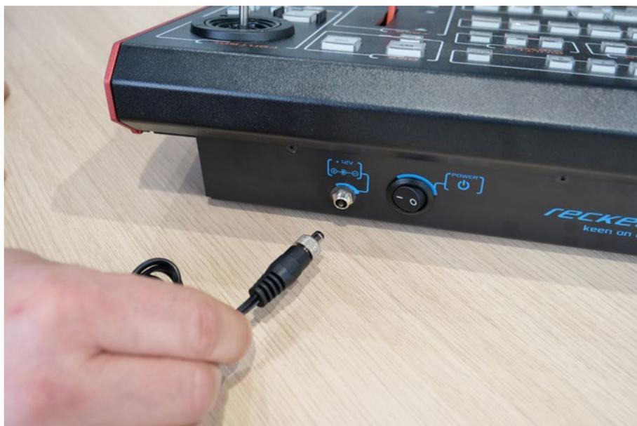
Next bolt the locking screw and connect the power supply unit to the electrical outlet. Picture below.
