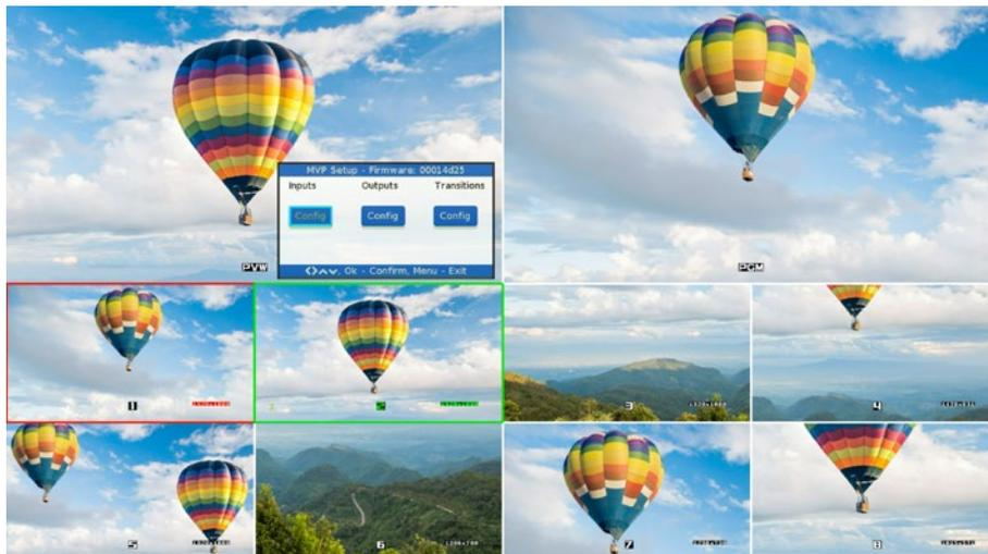
Press the MENU button and press the left arrow to navigate through the menu options until the "INPUTS" option is selected with a blue frame. Press OK to go to the next options.
