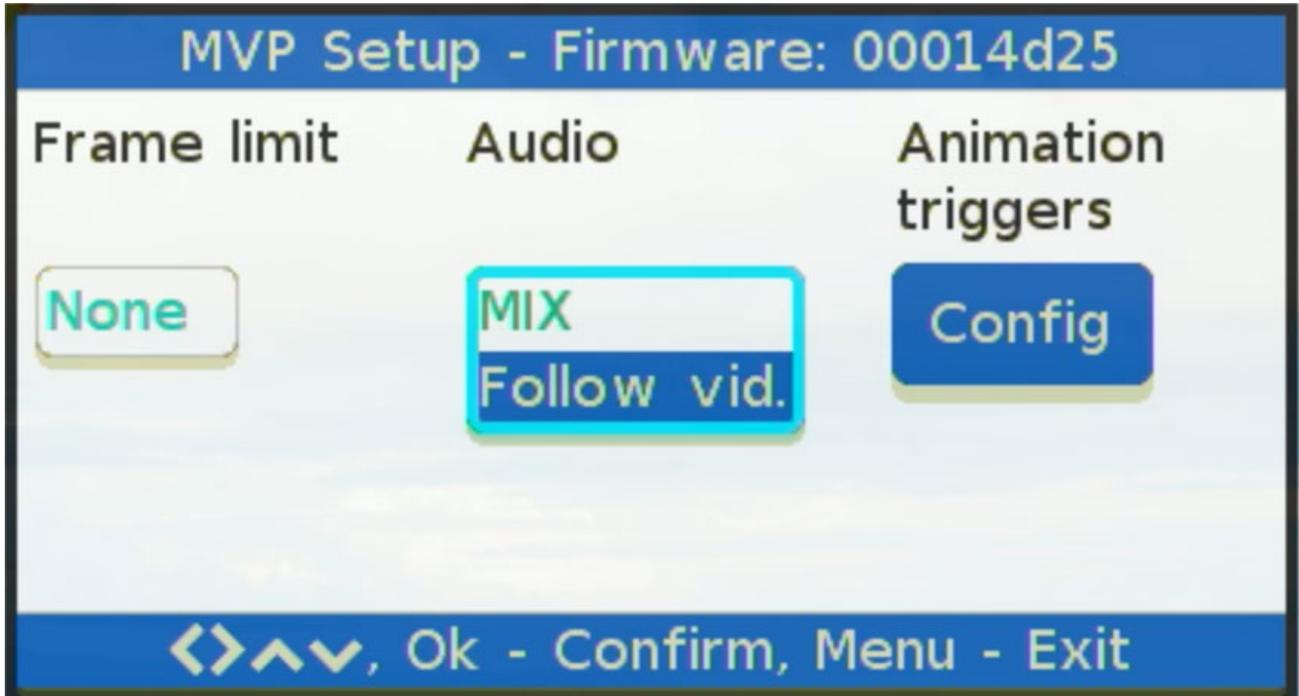
The "MIX" (mixing) function gives users the opportunity to hear the sound from both inputs A and B on the program output. The second one called "Follow Video" gives the user the opportunity to hear the sound depending on the button pressed in the Program line. On the SDI Aux output connector user always hear the own input. Frame 1 to 4, the audio from input 1 and 5 to 8 the audio from input 2. On the Multiviewer HDMI, there is always mixing all Inputs.
