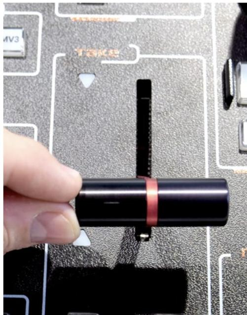
After several movements, all the LEDs will go out. This way, the keyboard has been calibrated and has returned to its normal operation mode.
