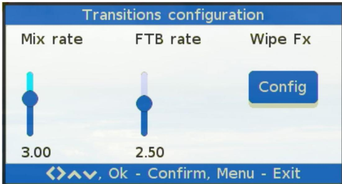
Instead of MIX effect it's possible to select on the MVP Keyboard the FX effect. Normal pressing switches transition to FX mode. After a long press, a popup will appear. User can define also a type of transition in WIPE fx menu.
